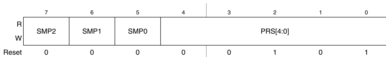
Figure 15-7. ATD Control Register 4 (ATDCTL4)
