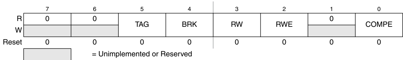
Figure 8-15. Debug Comparator Control Register DBGCCCTL (Comparator C)
