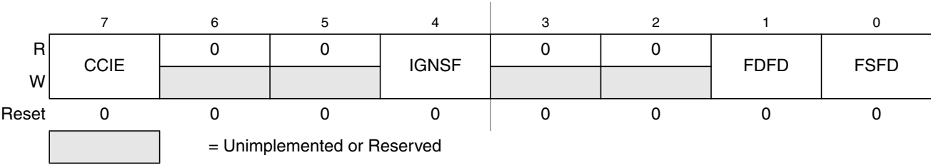
Figure 30-9. Flash Configuration Register (FCNFG)
