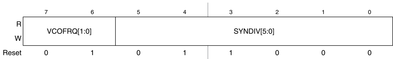
Figure 10-4. S12CPMU Synthesizer Register (CPMUSYNR)
